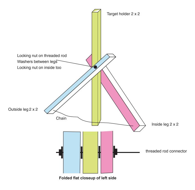
Leg length is adjusted so that Prone target is 500-700 cm above firing line
